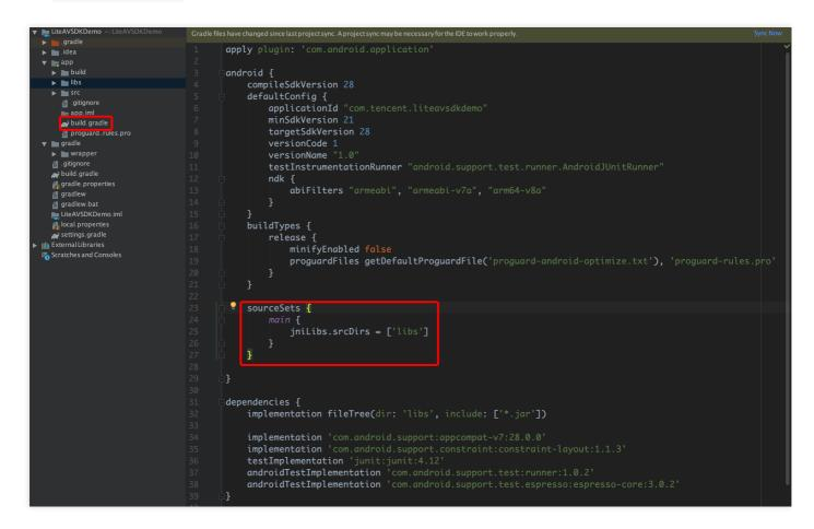
In defaultConfig of app/build.gradle , specify the CPU architecture to be used by the application.
