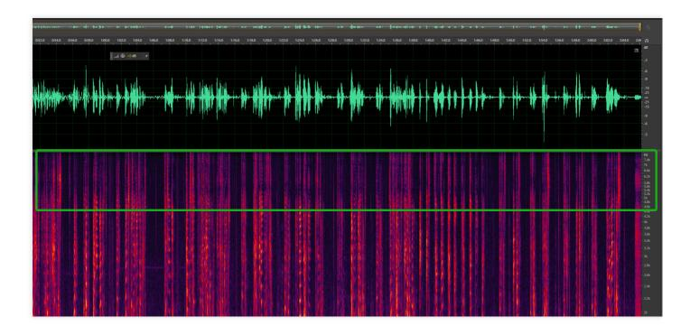
The waveform and spectrum of a fake 16,000 Hz audio is as follows (which is actually 4.6 kHz  $^*$  2 = 9.2 kHz). It can be seen that the audio information is completely missing in the 4.6k–8k frequency band.
