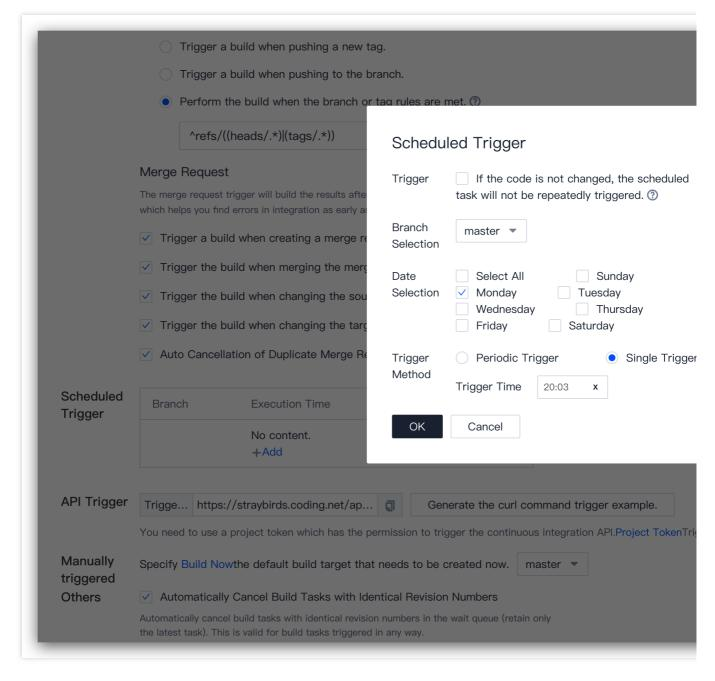
Trigger condition: Do not repeatedly trigger scheduled task if code is unchanged
