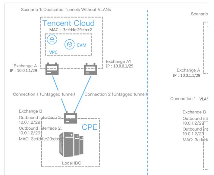
As shown in the figure above, customer exchange B connects to Tencent Cloud exchanges A and A1 through two connections (connections 1 and 2).
