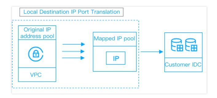
Local source IP port translation only supports access requests initiated by resources in a VPC. To access ports within the VPC via Direct Connect, the IDC should also be configured with local destination IP port translation. For local source IP port translation, access requests initiated by resources in a VPC are stateful connections. Therefore, response packets are not a concern.
