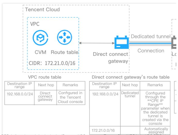
For a BGP dedicated tunnel, the destination IP range of IDC routes to a Tencent Cloud VPC is the VPC CIDR block ( 172.21.0.0/16 ) obtained by the local router based on the BGP protocol.
