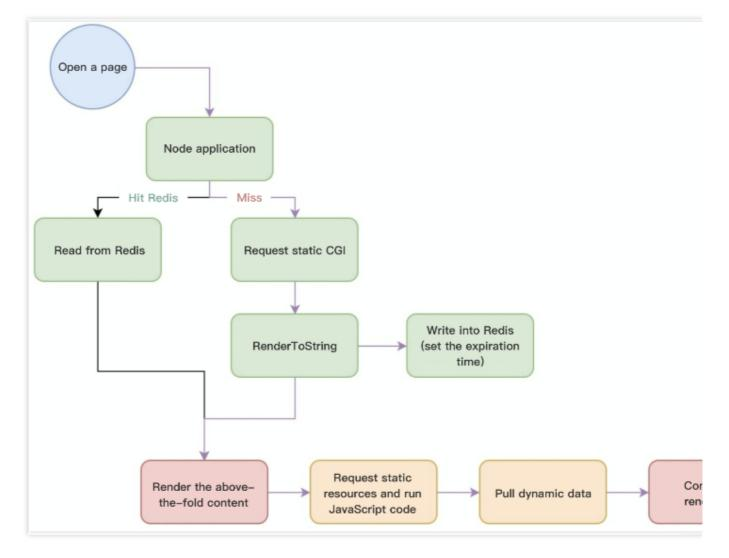
Redis is used to cache the page rendered with static data, which not only accelerates SSR rendering but also improves the QPS of a single server (renderToString is a CPU-intensive operation in a certain sense).
