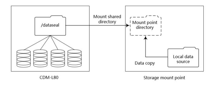
After receiving a CDM-L80, you need to locally mount the shared directory /dataseal in it to perform data copy. (It is recommended that each bucket be a separate folder directory named after the bucket name.)
