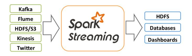
Spark Streaming abstracts continuous data into a Discretized Stream (DStream), which consists of a series of continuous resilient distributed datasets (RDDs). Each RDD contains data generated at a certain time interval. Processing DStream with functions is actually processing these RDDs.
