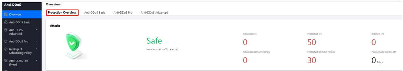
2. In the "Attacks" module, you can view the application security status, the latest attack and the attack type. To obtain higher protection, you can click **Upgrade Protection**.
