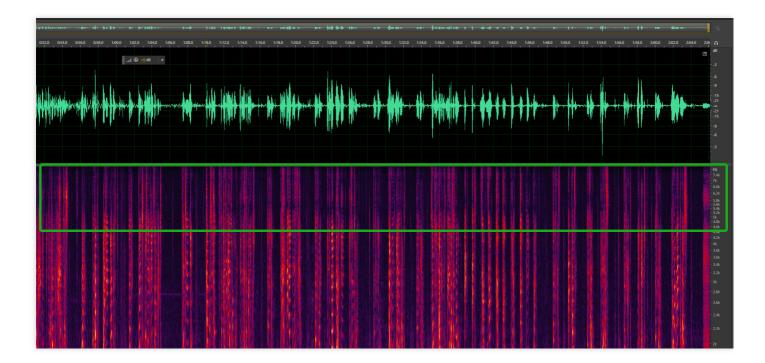
The waveform and spectrum of a fake 16,000 Hz audio is as follows (which is actually 4.6 kHz \* 2 = 9.2 kHz). It can be seen that the audio information is completely missing in the 4.6k–8k frequency band.
