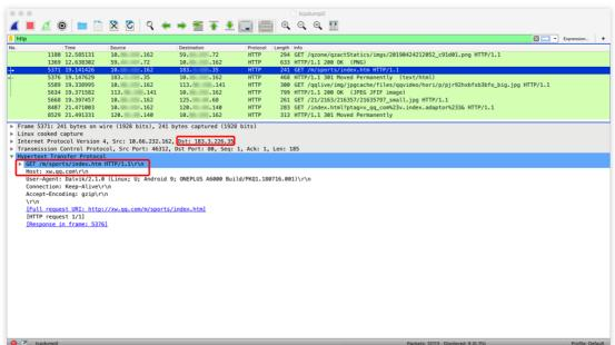
From the perspective of packet capture, the request for xw.qq.com is eventually sent to the server at the IP address 183.3.226.35 .
