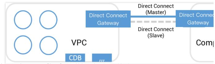
**VPN connection** serves as Direct Connect Linkage slave (master/slave).
