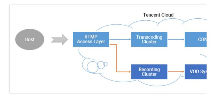
After you enable recording for a live stream, each audio/video frame published from the host's mobile phone will be relayed to the recording system and written into a recording file.
