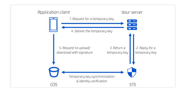
As shown in the figure above, the user has developed the app client, and the permanent key is stored in the user server. The following steps are required to use a temporary key for frontend direct upload:
