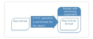
If there are versioned objects in the bucket, the objects newly uploaded to the bucket will become the current version with a version ID of null as shown below:
