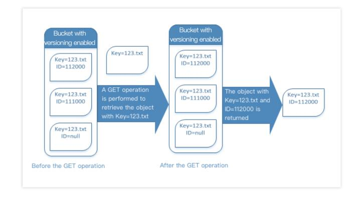
A GET request with a version ID specified returns the specified version of an object. The following figure shows how such a request returns the specified version of the object. The request can also return the current version.
