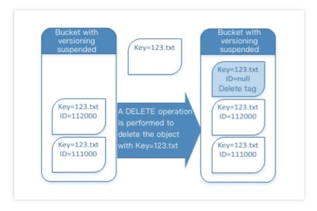
Even in a bucket where versioning is suspended, the root account is still able to delete a specified version permanently.
