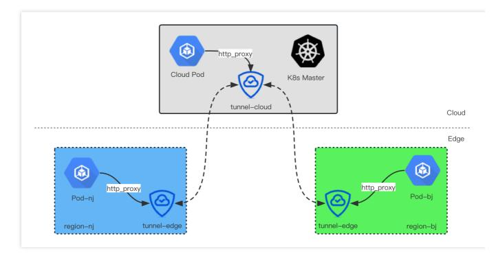
As illustrated in the diagram above, the edge node tunnel-edge will establish a bidirectional tunnel with the cloud tunnel-cloud. The tunnel-edge will open the local 8080 port as the http/https proxy port. If an edge Pod needs to access other regions' Pod IPs or services through a proxy, you can specify the http\_proxy or https\_proxy environment variable within the Pod. This will forward the http/https traffic through the tunnel to the cloud or other edge nodes in different regions.
