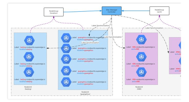
For example, you can classify the nodes in the cluster according to two types of scenarios based on your requirements. One scenario is by location, and the other scenario is by architecture. Each scenario represents a NodeGroup Custom Resource (CR) instance - location and arch. Then, you can add different NodeUnits to the corresponding NodeGroup categories.
