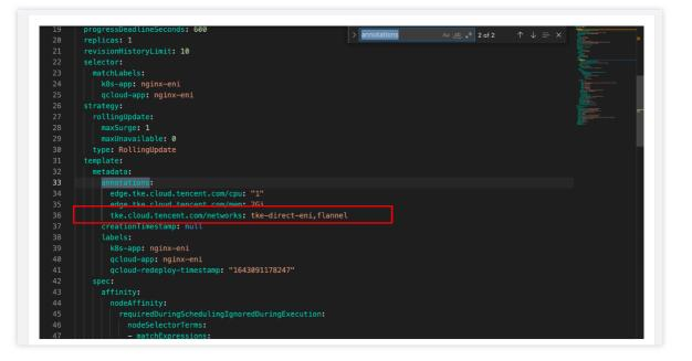
The ENI capability of edge clusters is supported only by Tencent Cloud CVM node resources. Therefore, when deploying an application, you need to use the nodeAffinity capability to schedule the Pod mounted with the ENI to the real CVM edge node (you can enter multiple CVM node IDs).
