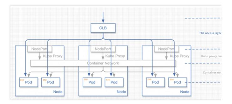
You can also use ENIs in the VPC where the CVMs reside to open Pods to external users and then bind different ENIs to the CLB to enable high-performance network forwarding.
