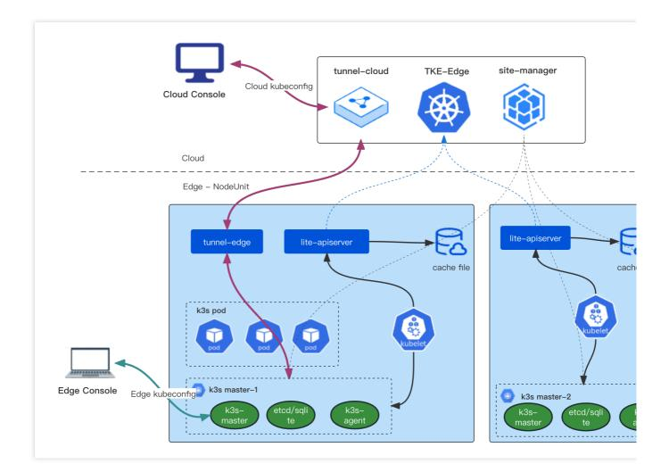
For example, the three edge nodes can be divided into a NodeUnit. Through edge node pool-related operations, the K3s master and agent components can be deployed on these three nodes to form an independent single-master or 3-master K3s cluster. This edge K3s cluster can be accessed from the cloud via a tunnel, and it can also be accessed directly on the edge-side nodes.
