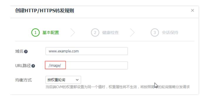
After the forwarding rule is created, you can see that forwarding groups and forwarding rules have been configured for www.example.com/image/ under the listener. Then you can click **Bind CVM** to select the CVM for which we have just configured the service. When binding CVM, the backend port 80 is set as the default listening port. The configuration of application-based cloud load balancer is flexible, so you can bind CVMs of different backend ports under the same listener.
