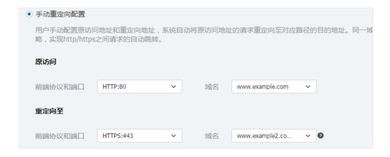
Click **Next** to select the original and redirected access paths. If there are many paths under the domain name, you can add multiple paths for redirection. Note: The path configuration does not allow loopback (that is, A-> B B-> C), and the configuration can only be performed in the same LB instance for now.
