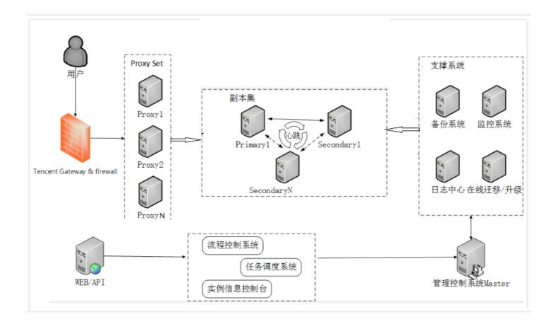
In the replica set architecture, the system automatically builds a "one master, two slaves" architecture. If the business expands, you can expand the computing or storage resources of each node.
